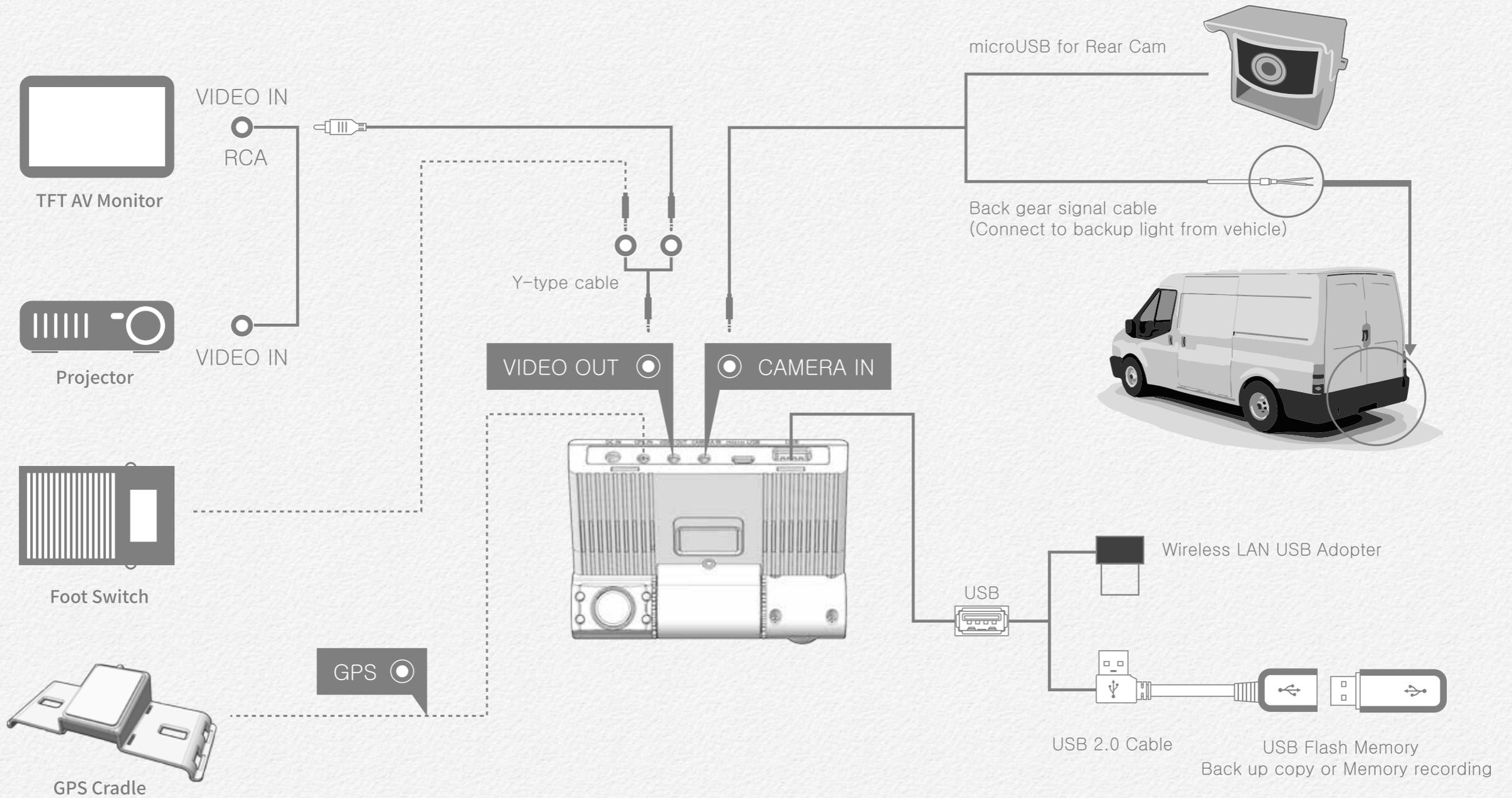
All the devices are must be connected to each port before supply the power to main NDR.
