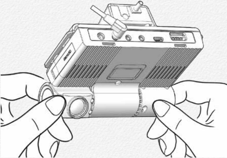
2) Fit tamperproof cover's hook to camera angle's hole after adjust camera angle.
