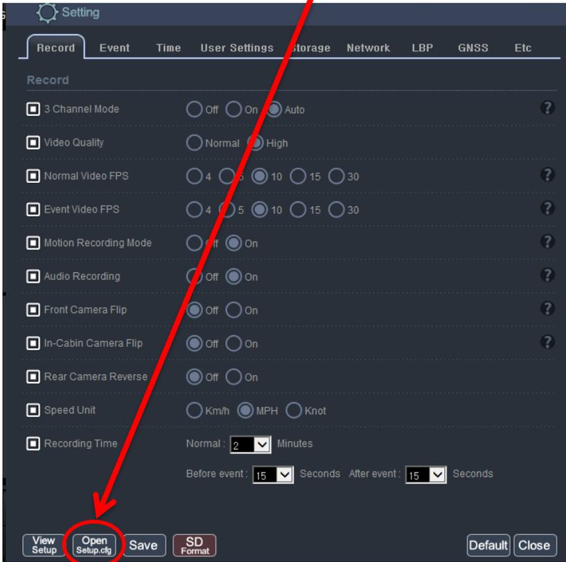
4. Select the USB Drive and Select the setup.cfg / setup from the open box, then click OPEN
