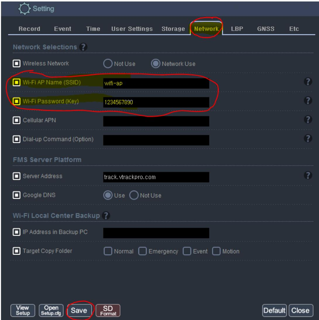
6. Click Save after finished all the config to save the new configuration to SD card. Over-write the save file and you should see “CFG File Saved” message
