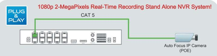
TRUE PLUG & PLAY IP SYSTEM! No IP setup necessary, all cameras POE (Power Over Ethernet)! 1080P Display, Smart Phone Support, EZ CMS Available with Analog DVR + HDSDI DVR + IP NVR
